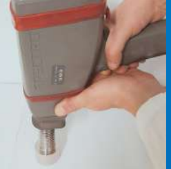
Hot-dip galvanizing thickness control
